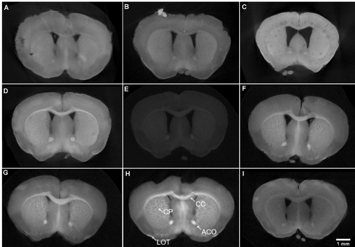
Figure 6: Comparison of the coronal sections of mouse brain samples selected from the original publication (Zikmund et al. , 2018). The compared images of differently contrasted brains are shown with the same histogram setting (possible due to the batch scan of all samples together). The contrasting protocol H (1% iodine in 90% MeOH for 24h) was determined as a best contrasting solution based on the analysis of obtained data, it had efficiently visualized the caudoputamen (CP), anterior commissure (ACO), corpus callosum (CC) and lateral olfactory tract (LOT).
