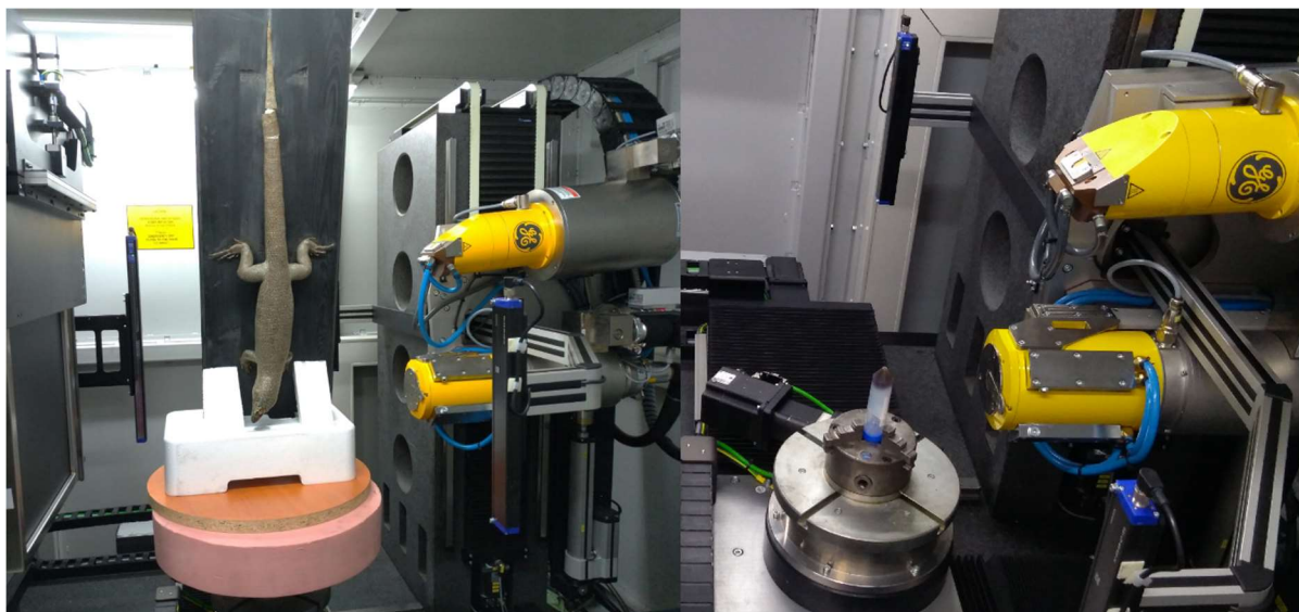
Figure 5: Motion stabilization of different kinds of samples, on the left is taxidermied sample of ameiva lizard fixated in position by styrofoam, on the right mouse embryo in the falcon tube and agarose gel.
