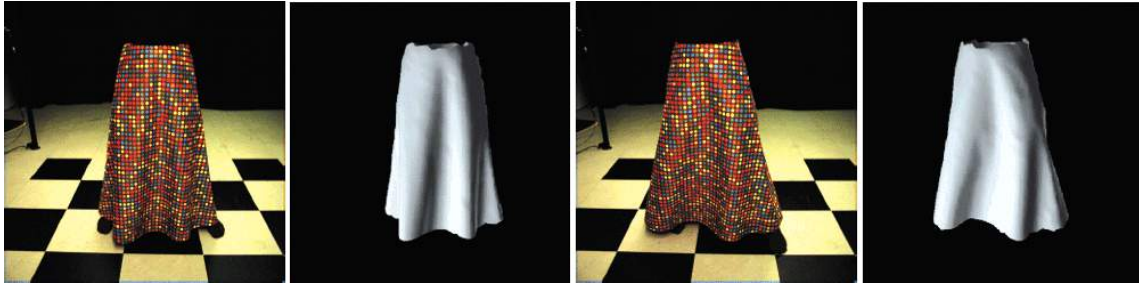
Figure 3.2: Pseudorandom array submaps printed on cloth with 3D reconstructions of the models [144].
