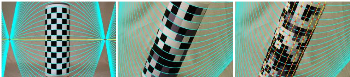
Figure 3.22: Detection algorithm for Uniform Marker Fields mapped on a cylinder [71]. Left: approximation of ellipses forming the rings on a cylinder with parabols coincident with two common points on the horizon. Center: detected pencil of parabols. Right: detected module centers on the cylinder.
