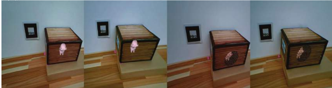
Figure 2.23: Augmenting virtual object behind a real surface. Left side image pair shows the pig inside the box without depth hints and the right image pair shows improved depth perception with „stereoscopic pseudo-transparency“ [118].
