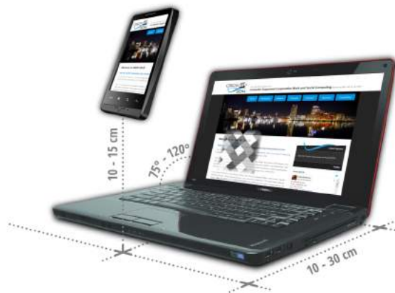
Figure 5.11: Parameters of marker detection reliability setup – distance between mobile device and laptop, range of screen angles used during tests and height range of a mobile device in order to be focused on the same point on screen.
