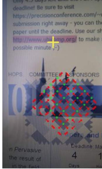
Figure 5.6: A successfully detected Uniform Marker Field as seen by the requester device’s camera with a crosshair shown to aid the user with targeting. The purple highlight is the content provider’s reaction to targeted content based on continuous interaction.
