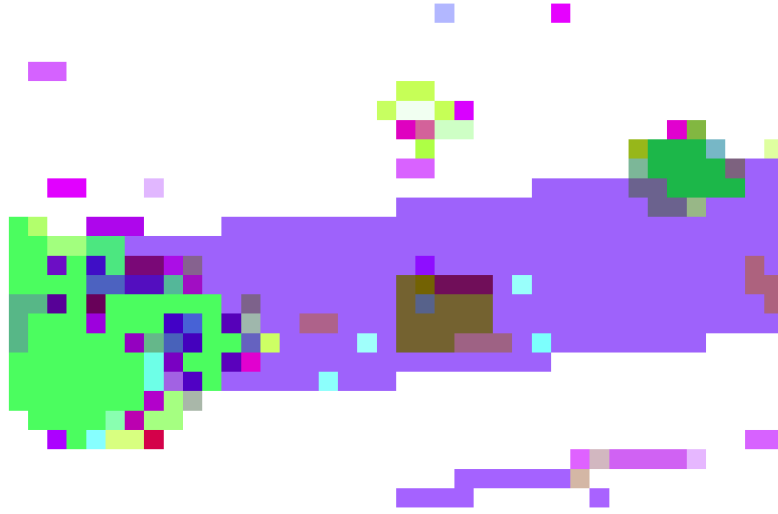
Figure 4.5: The segments used for finding the QR code. Red color component encodes the edge count per tile (inverted). Green color component represents the angle of the first dominant direction ( \alpha_1 ). Blue color component indicates the absence of the QR code based on p (refer to Equation (4.1)).
