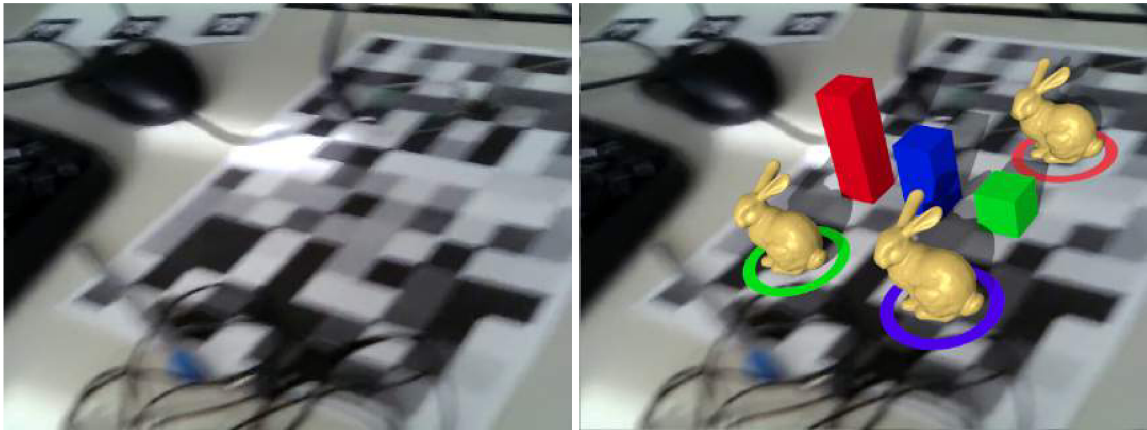
Figure 3.17: Result with grayscale Uniform Marker Field. Marker Fields with clutter, occlusion, varying lighting, strong blur. left: Original image – input to the recognizer. right: Recognized camera location and augmented scene.
