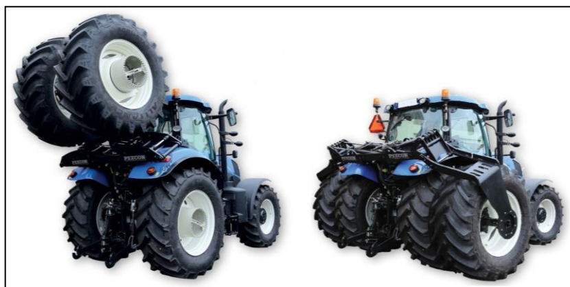
Obr. 26 Systém Gull Wing Double Tyre (www.peecon.com)
