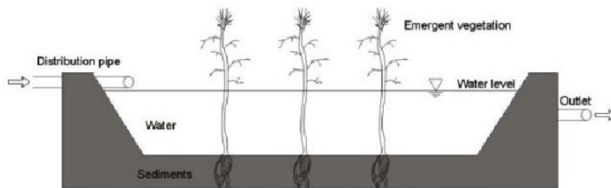
Figure 3: CW diagram with surface flow (Langergraber et Haberl 2004).
