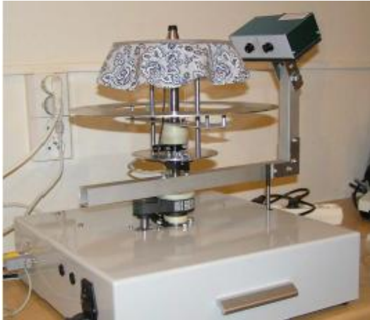
Obr. 3 3D drape scanner [17]
