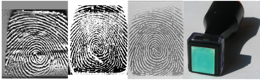
Figure 3.2: Stamp captured by different types of sensors [40]: left fingerprint - thermal sensor (Bergdata FCAT 100), middle fingerprint - optical sensor (Suprema SFM3020-OP), right fingerprint - capacitive sensor (Suprema SFM3050-TC1). Right picture: Picture of stamp of fingerprint.
