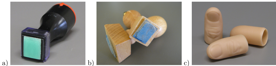
Figure E.1: Stamps and prosthetic fingers used for sensor spoofing.
