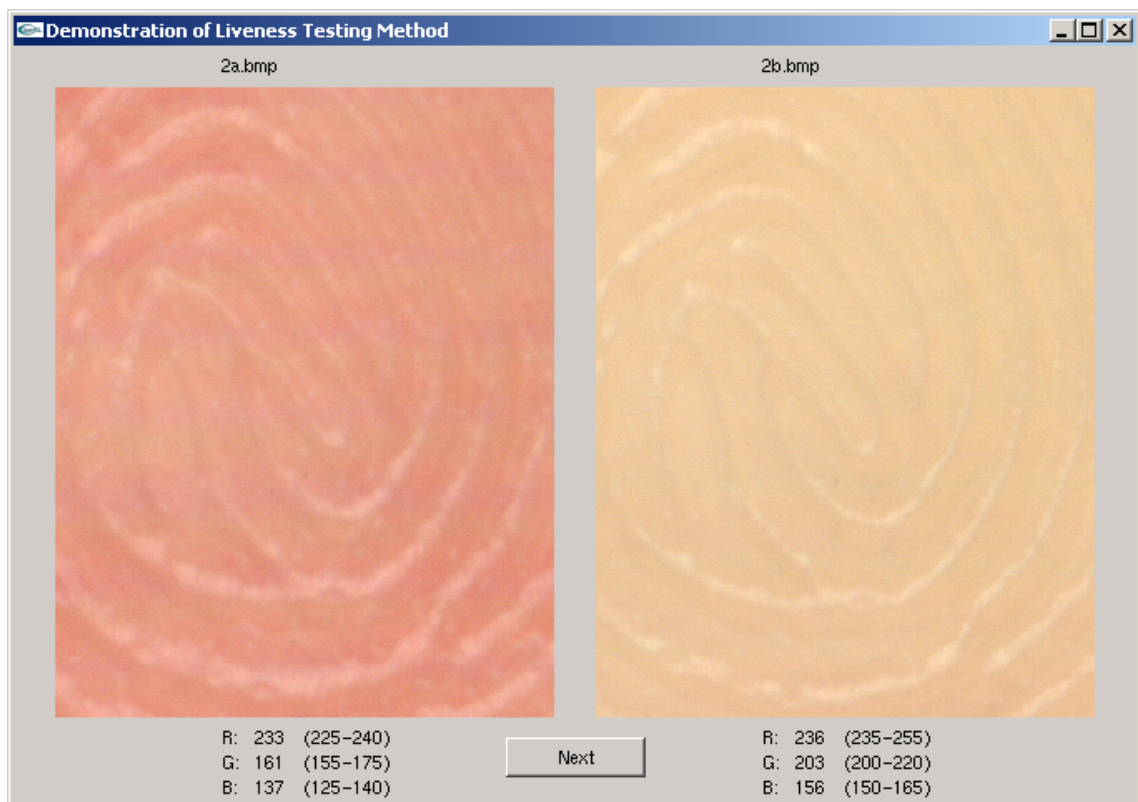
Figure D.1: Determining the color change: Loading two fingerprints (image before and after pressing) and determining the median of RGB components for each image.
