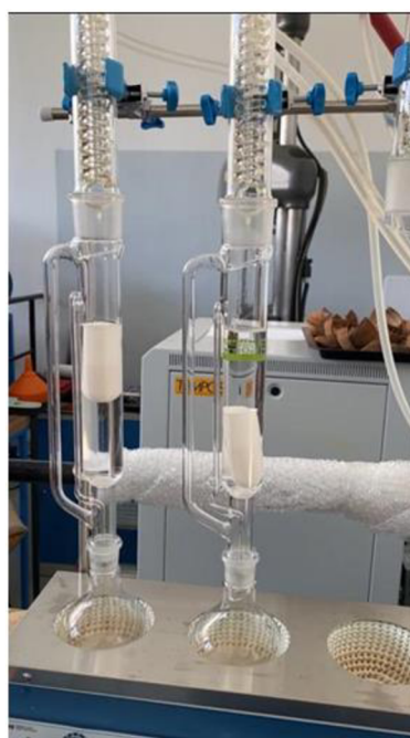
Figure 3. Soxhlet extraction procedure for the determination of sample oil content.
