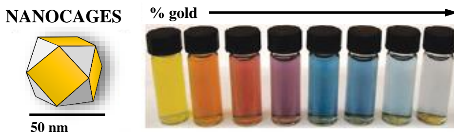
Fig. 3 – The percentage of gold in nanocage solution related to colour (Dreaden et al. 2012).
