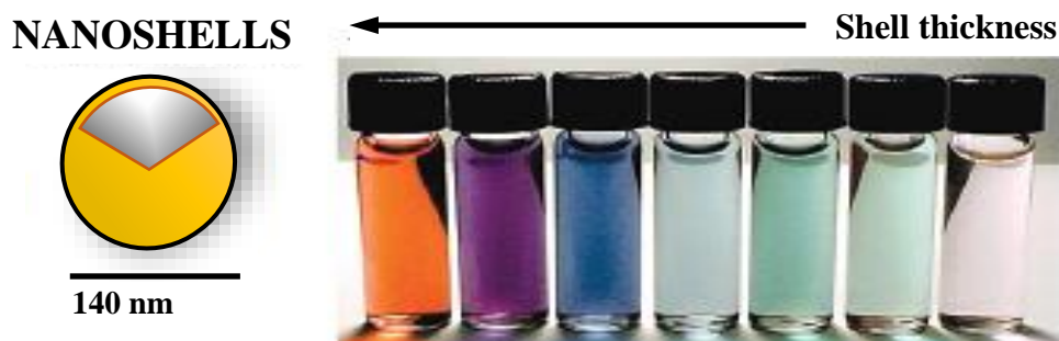
Fig. 2 – The shell thickness related to the colour of the silica-gold nanoshells (Dreaden et al. 2012).
