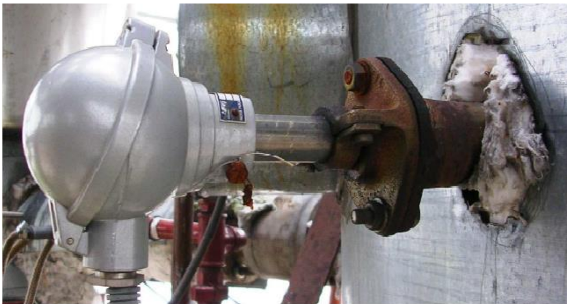
Figure 19 : Location of one of the rod thermocouple (type K)
