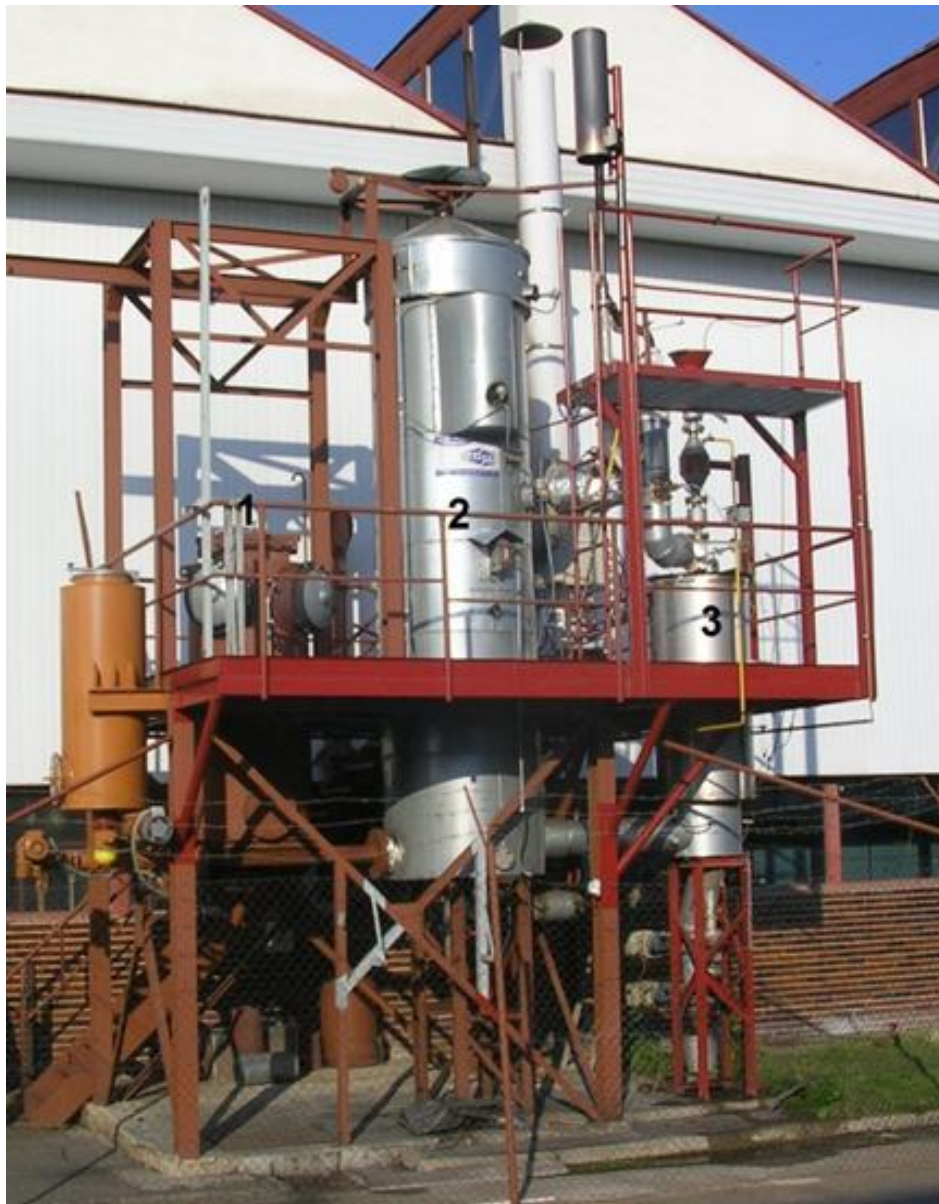
Figure 13 : Atmospheric fluidized bed gasifier Biofluid 100
