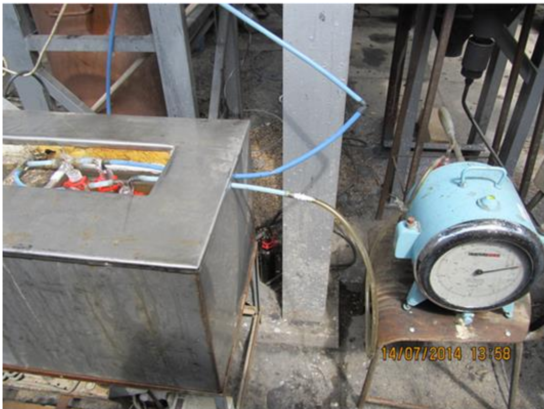
Figure 36 : The experimental equipments which used to measure tar content in a produced gas.
