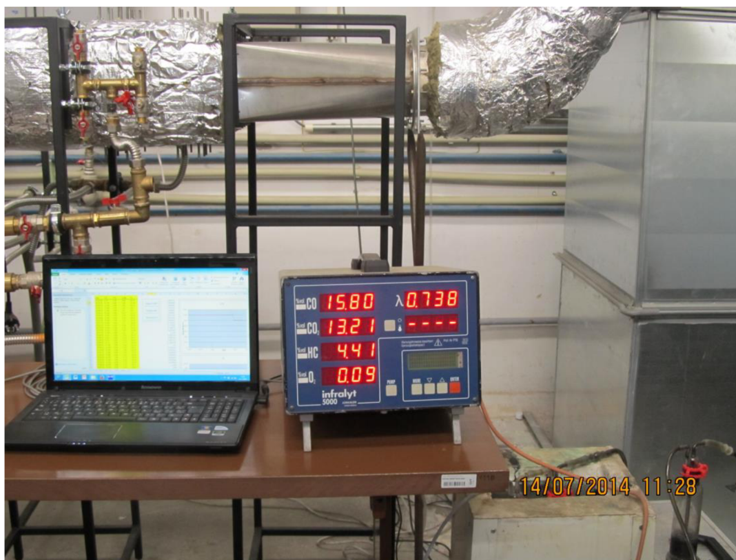
Figure 22 : Device INFRALYT 5000 for on-line evaluation of the basic components of produced gas
