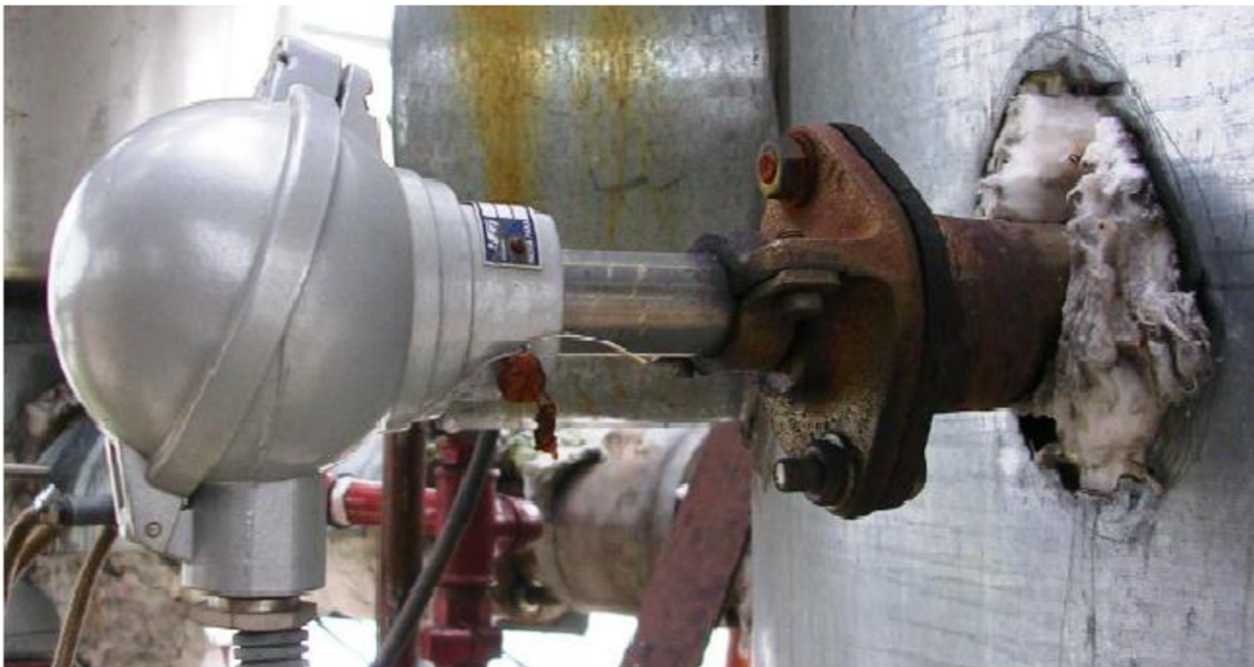
Figure 19 : Location of one of the rod thermocouple (type K)
