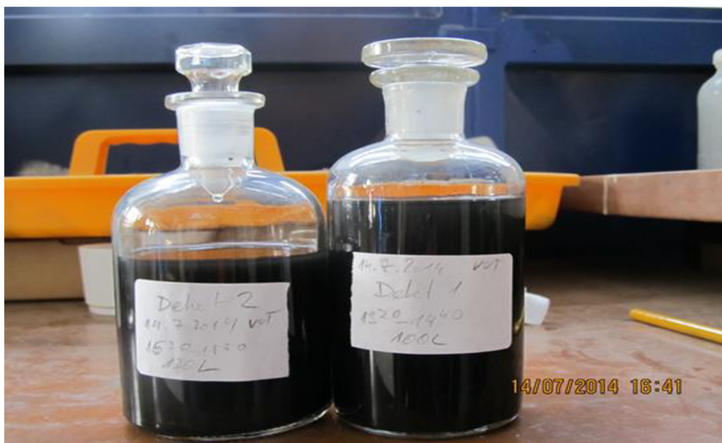
Figure 37 : The samples of tar which had been collected during the experiment
