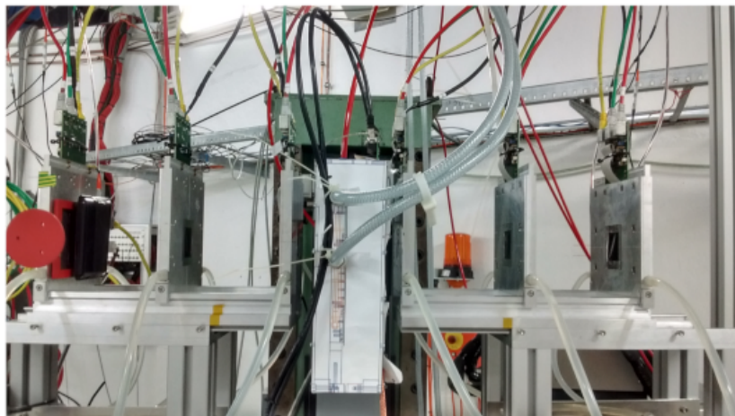
Figure 9: The DURANTA telescope at DESY, the central box houses the DUT. From [6].
