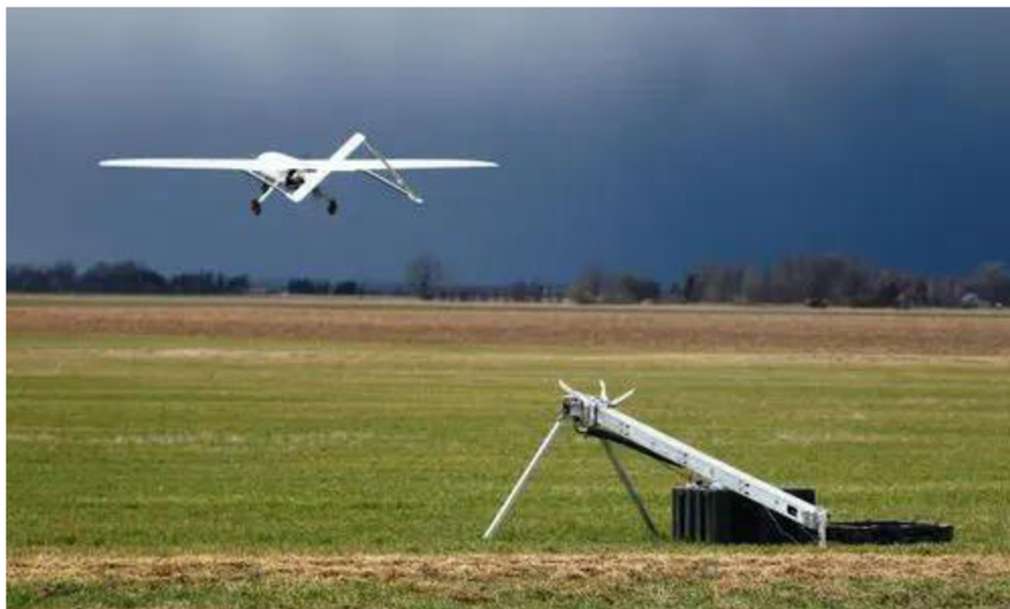
Figure 1. Pneumatic catapult for UAVs Reprinted from https://www.aeroexpo.online/prod/uav-factory-ltd-europe/product-174156-61637.html .
