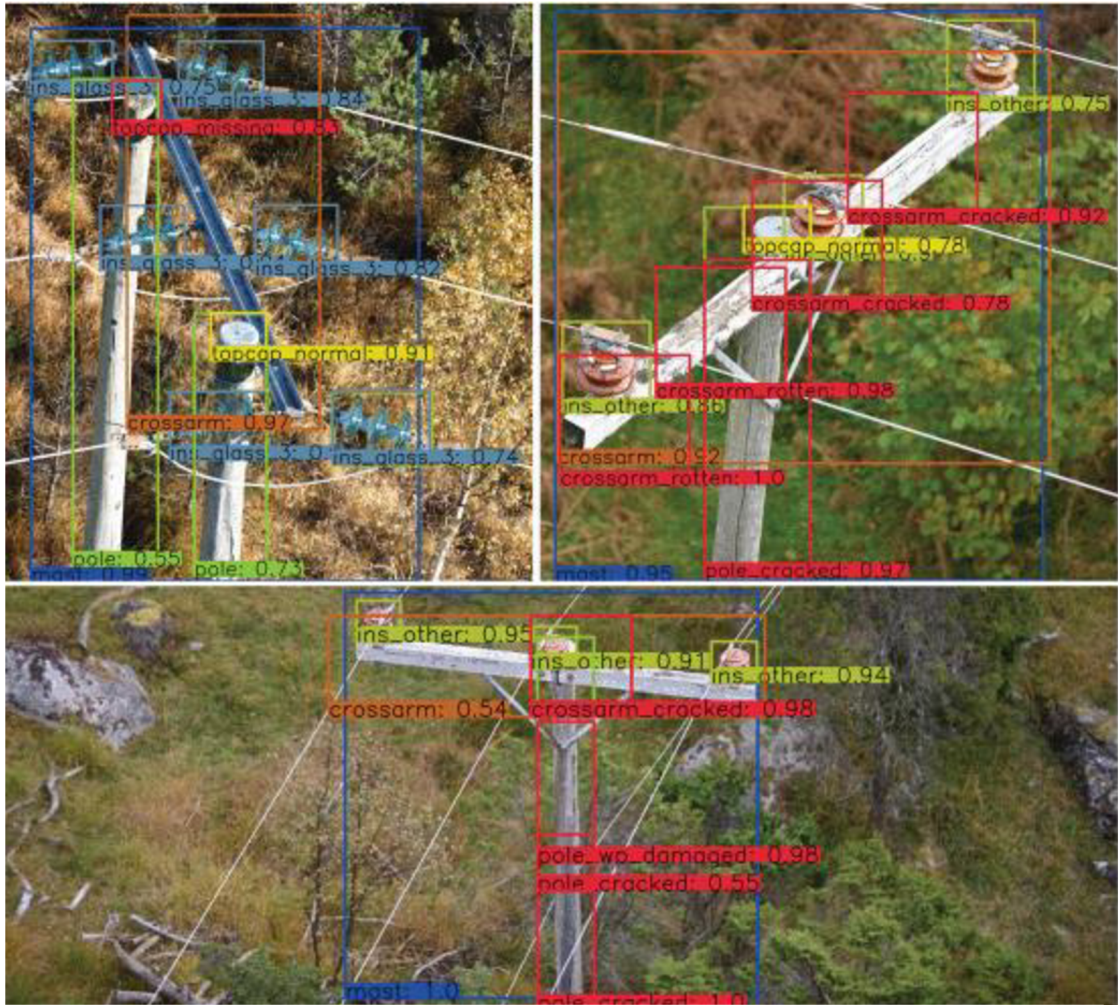
Figure 3. Output of machine-learning algorithm on top of UAV visual footage. Reprinted from Jenssen, R., & Roverso, D. (2019, p. 19)
