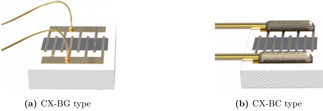
Figure 2.7: Two types of bonding of wires to both contact pads of the Cernox® thin film resistance cryogenic temperature sensors. In Figure (a), CX-BG type with the wires made of gold. In Figure (b), there is CX-BC type with the wires made of copper. Adapted from [17]
