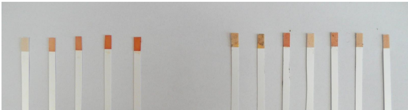
Figure 17: Comparison of samples with the colour scale of the standard solutions, blank, class 0, 1, 2 ,3, Tanja, Dejan, Oma, Maria, Ulrike, KiGa, Herta
