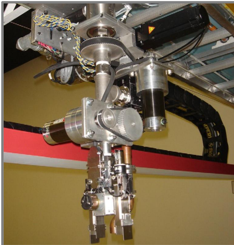
Obr. 2-4 Tisková hlava - metoda contour crafting [6]
