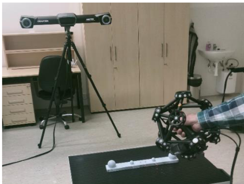
Figure 41: Scanning using METRA-scan (C – Track and Laser Head)
