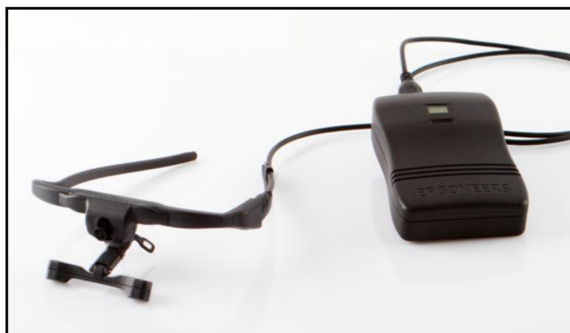
Obr. 12: Eyetracker Dikablis Glasses [37]
