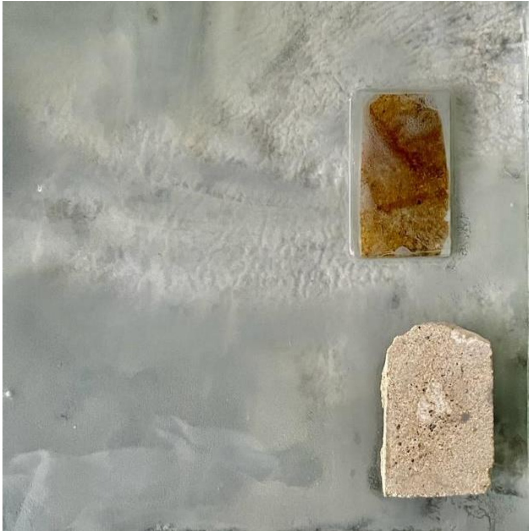
Figure 5 thin section sample grinded with glass plate and powder
