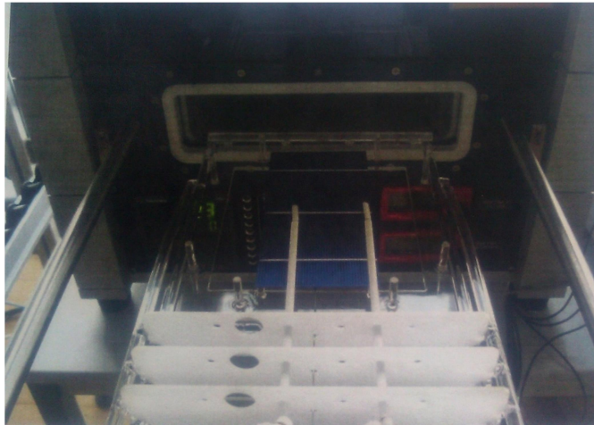
Fig. 66: RTP furnace modified for in-situ resistance measurement.
