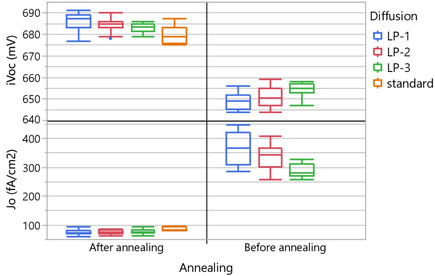
Fig. 40: iV_{OC} at 1 sun and J_0 of the cell precursors (before metallization) before and after annealing. The J_0 was extracted at an injection level of \Delta n = 2 \cdot 10^{15} cm^{-3} .
