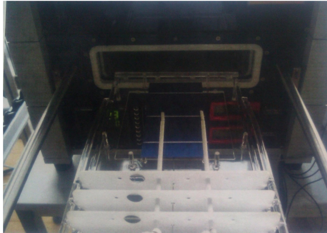
Fig. 66: RTP furnace modified for in-situ resistance measurement.
