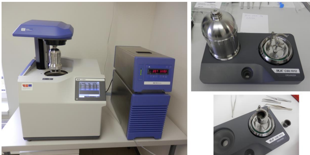
Figure 12 Calorimeter IKA C 6000 (left) and laboratory equipment (right)
