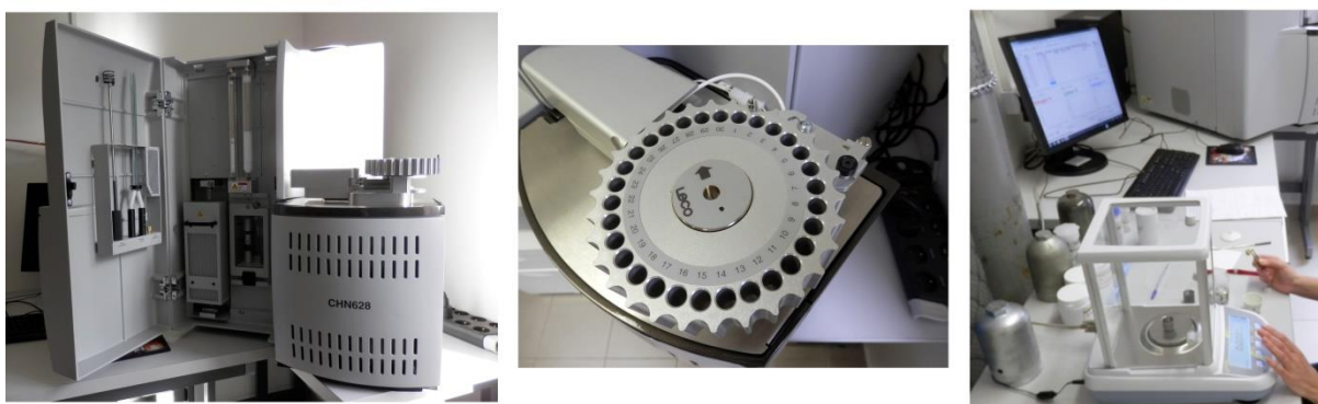
Figure 11 Leco (model CHN628) and preparation of samples (on the right side)
