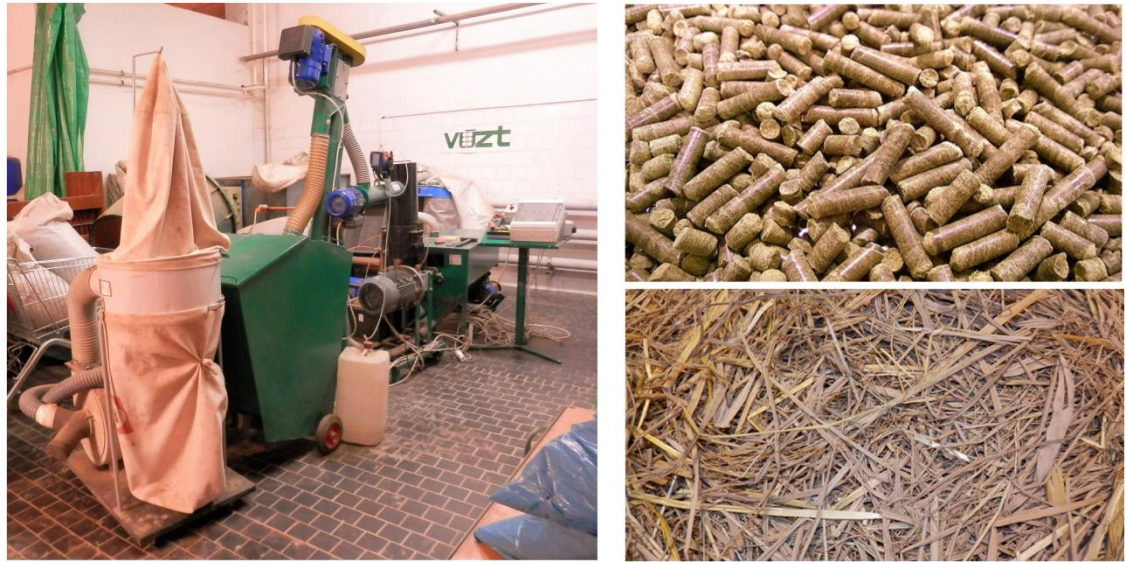
Figure 7 Pelletizer (left), feeding material and pellets (right)
