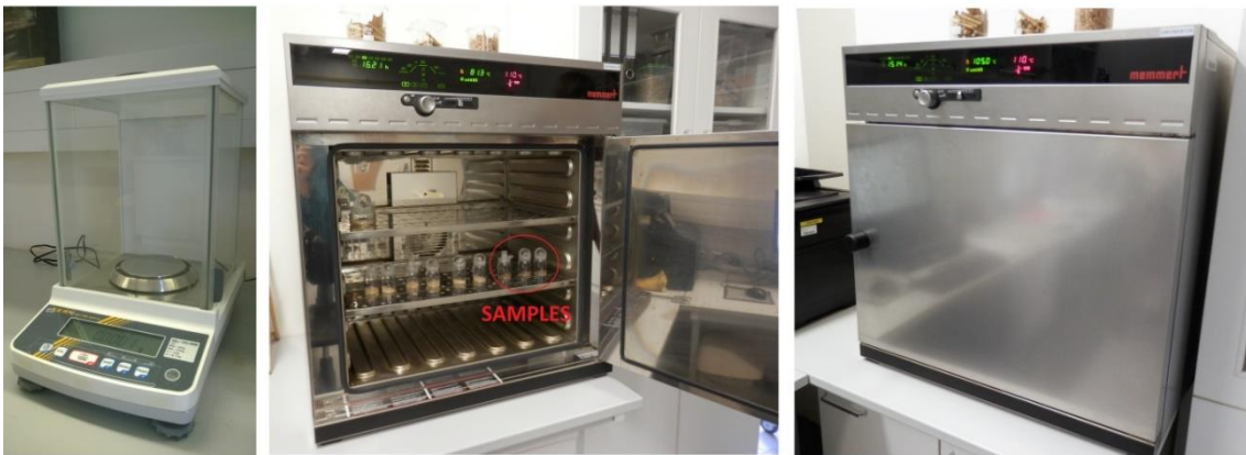
Figure 9 KERN Laboratory scale (model ABJ 120-4NM) and MEMMERT oven (model UFE 500) with samples
