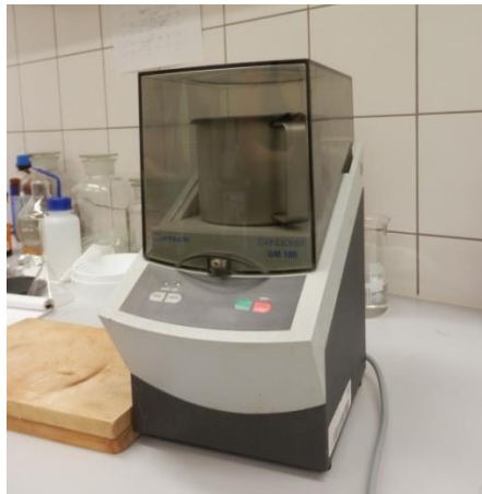
Figure 8 Retsch Grindomix GM 100 Grinding knife mill
