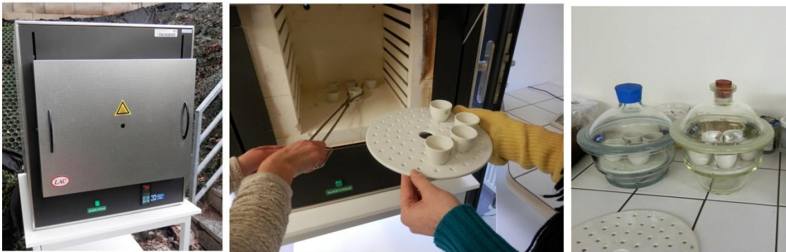
Figure 14 Muffle furnace and desiccator
