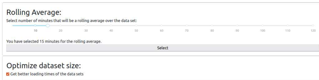
Fig. 3.15: Two added sections for averaging the static dataset and optimizing the loading time of the page
