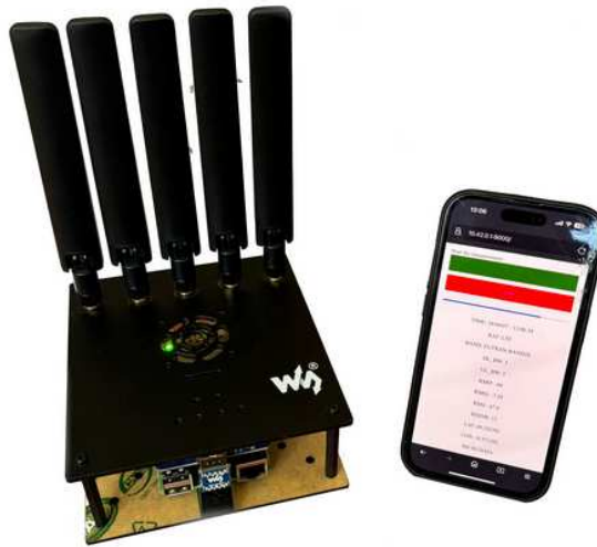
Fig. 1. Simcom SIM8200EA-M2 5G Module together with measurement setting application running on Raspberry Pi
