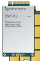
(a) Simcom SIM8200EA-M2 (b) Quectel RM500Q series (c) Sierra Wireless EM9190
