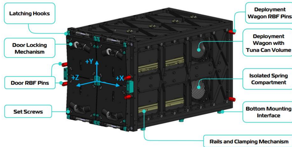
Figure 9 EXOpod 12U CubeSat Deployer [16]
