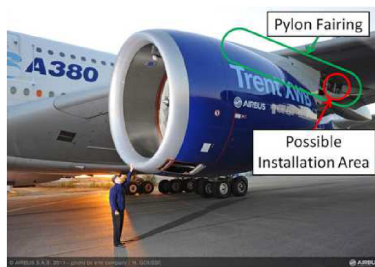
Fig. 5 Opportune spot for placing of TEG on the pylon fairing of Airbus A380 [13]
