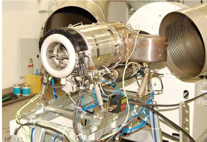
Fig. 10 TJJ100 turbine with JECU (black box in the rear section) on the test stand [20]
