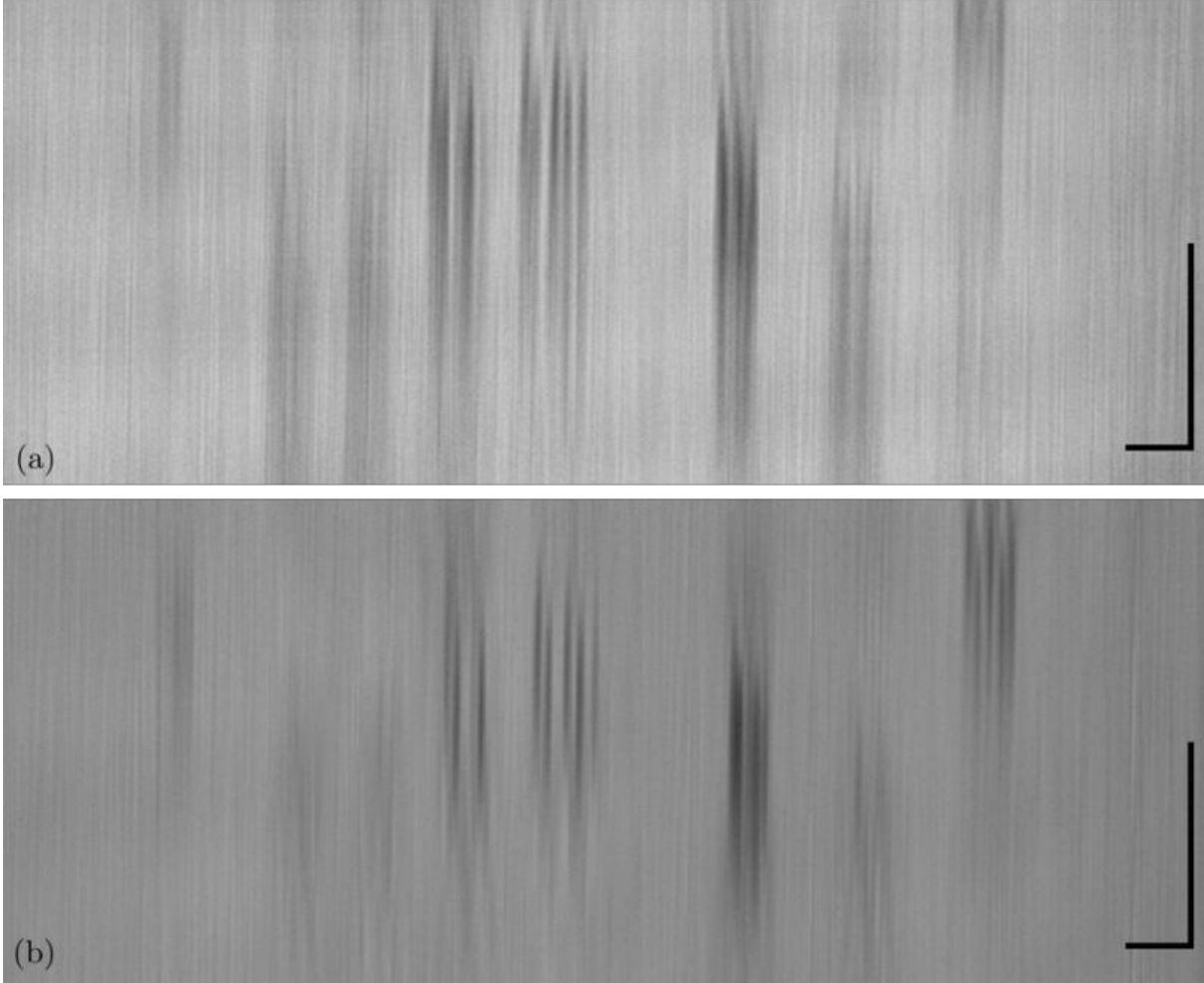
Figure 15: xz cross section of the whole hydrogel z -stack, (a) NA_S = 0.3 , (b) NA_S = 0.5 ; scale bars 10 \mu\text{m} ; numbers of the structures shown above.
