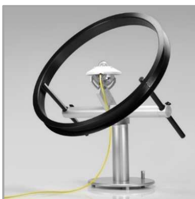
Obr. 27: Clona pro pyranometr [38]
