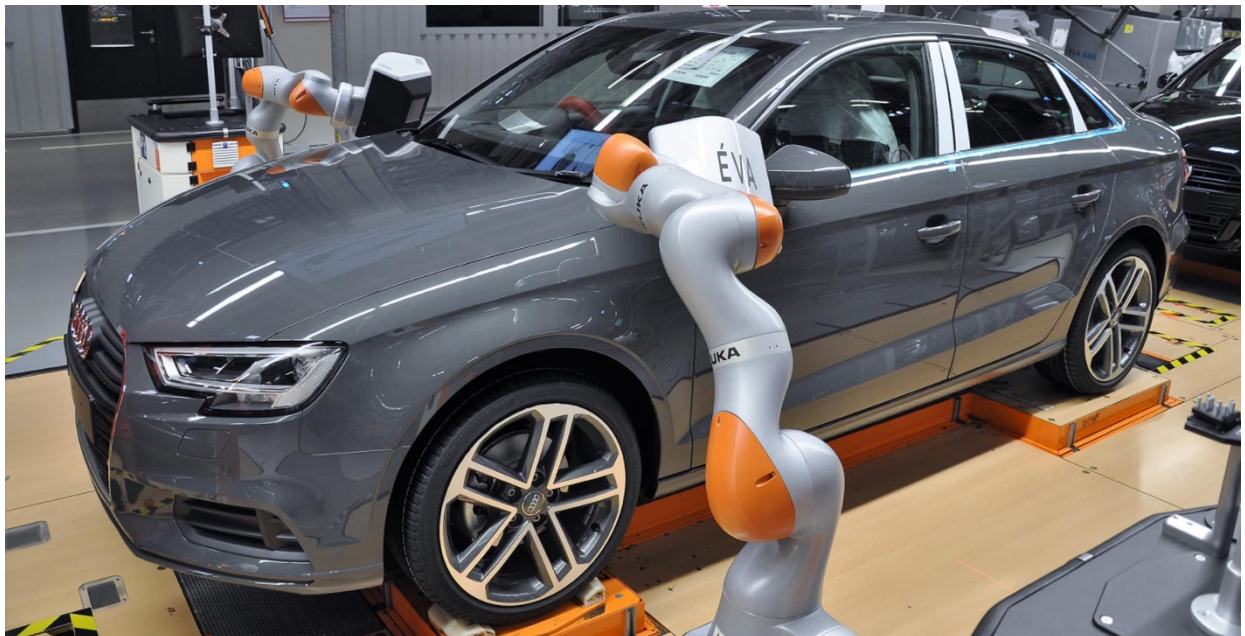
Figure 11 Optical Robotic arm EOL inspection
