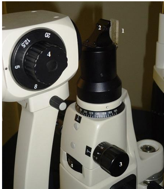
Obr. 13 Diffusing filter (1), mirror (2), control of the slit beam width (3), magnification zoom (4)
