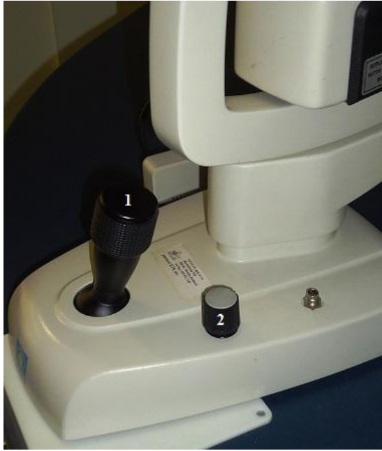
Obr. 12 Joystick (1), light intensity controller (2)
