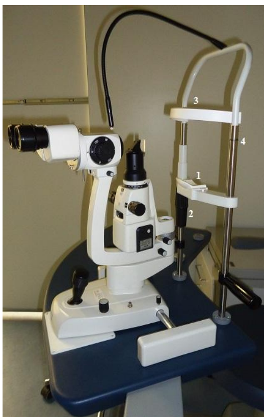
Obr. 11 Slit lamp – chin – rest (1), height controller (2), forehead – rest (3), Bar with lateral mark of height of the eyes (4)
