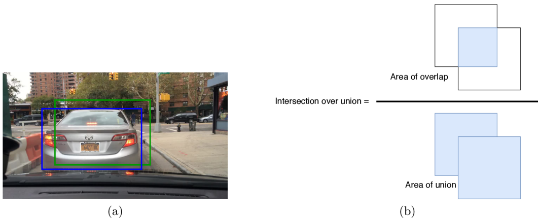
Figure 3.7: IOU is used to measure how much predicted bounding box overlaps with the ground truth bounding box. On Figure (a) ground truth rectangle (blue) overlaps predicted bounding box (green). Image is taken from BDD dataset [41]. On figure (b) is shown how IOU of two bounding boxes is computed.
