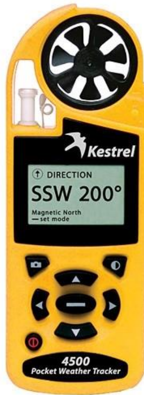
Figure 4. Kestrel 4500 Used to measure weather conditions.
