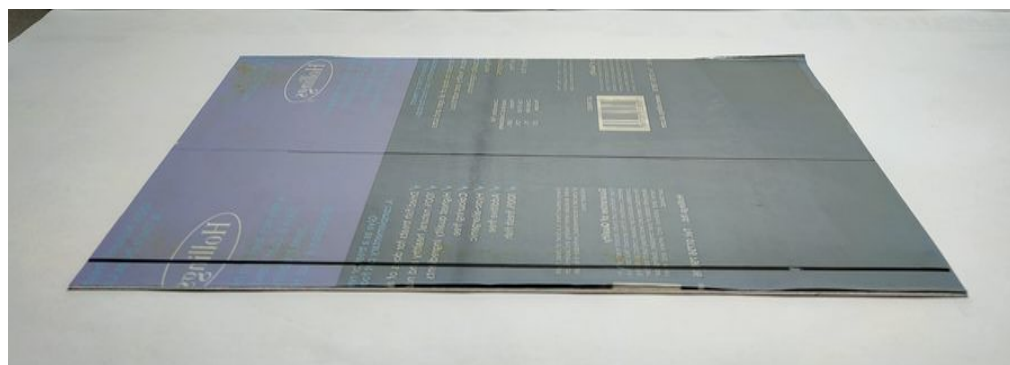
Fig. 4.22: LDPE packaging film covered with ND-P/PAA 100 F coating stuck to aluminum plate. Source: photograph by author.
