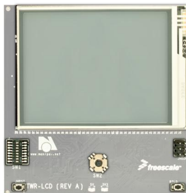
TWR-LCD: Graphical LCD Tower System Module
