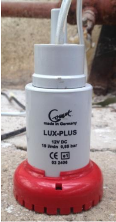
Figure 6: Water Pump (Photo: Author).
