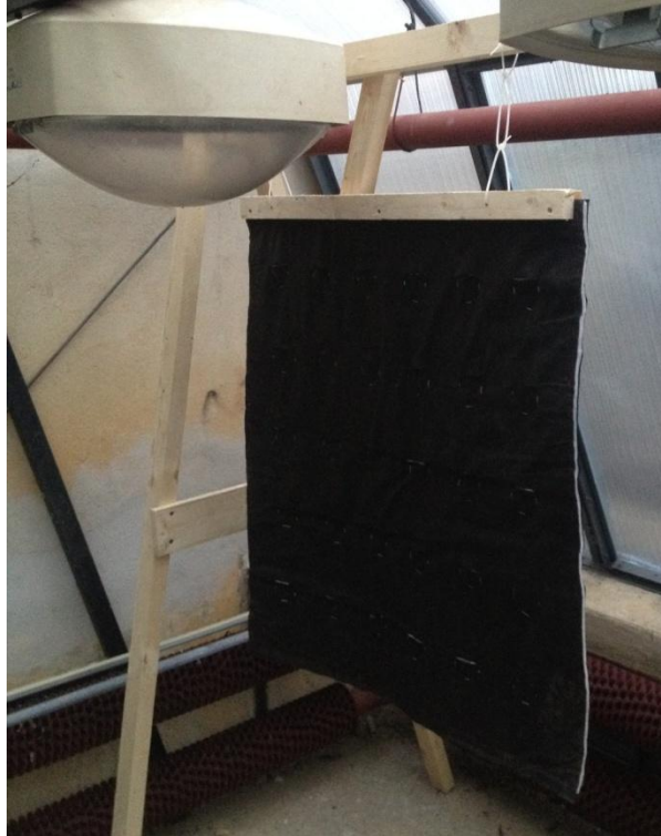
Figure 4.8: Wooden framework and hanging mechanism with complete wall panel attached (Photo: Author).
