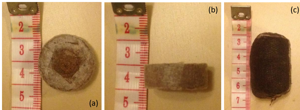
Figure 4.6: (a) Diameter of dry peat pellet. (b) Length of dry peat pellet. (c) Length of wet peat pellet (Photo: Author).
