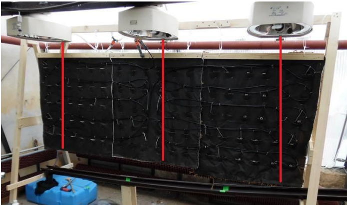
Figure 8: Location of light fixture. Red line indicates location on wall directly below the light bulb (Photo: Author).
