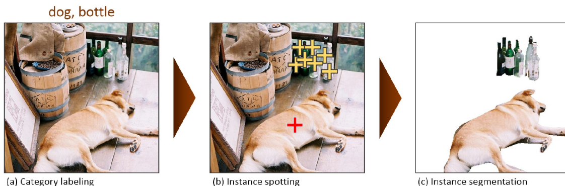
Figure 3.1: The MS COCO annotation pipeline, in sequence: (a) Labeling the categories present in the image, (b) locating and marking all instances of the labeled categories, and (c) segmenting each object instance. Taken from [LMB + 14]
