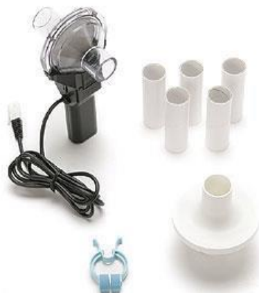
Obr. 10: Spirometr SPR - BTA
