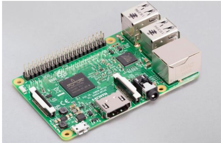
Obr. 23 RaspberryPi 3 Modul B [42]
