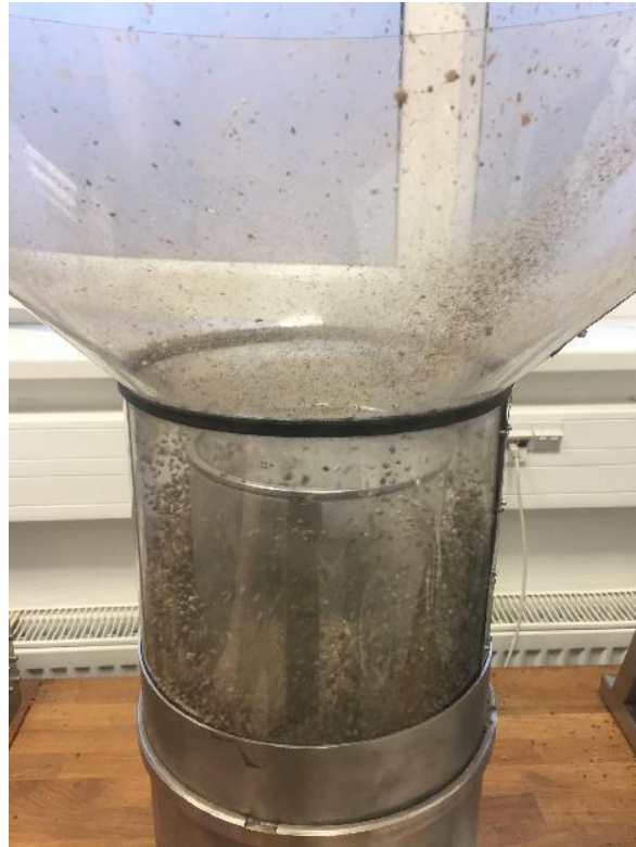
Figure 12. Cleaning of the seeds by Farnet ® air blower (Source: Author)
