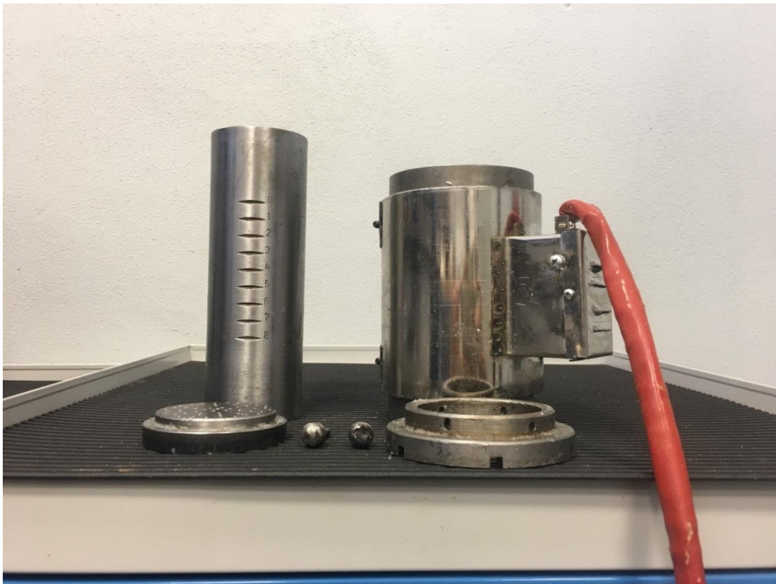
Figure 13. Disassembled metallic cylinder used for pressing (Notice the heating sleeve with the red wire) (Source: Author)
