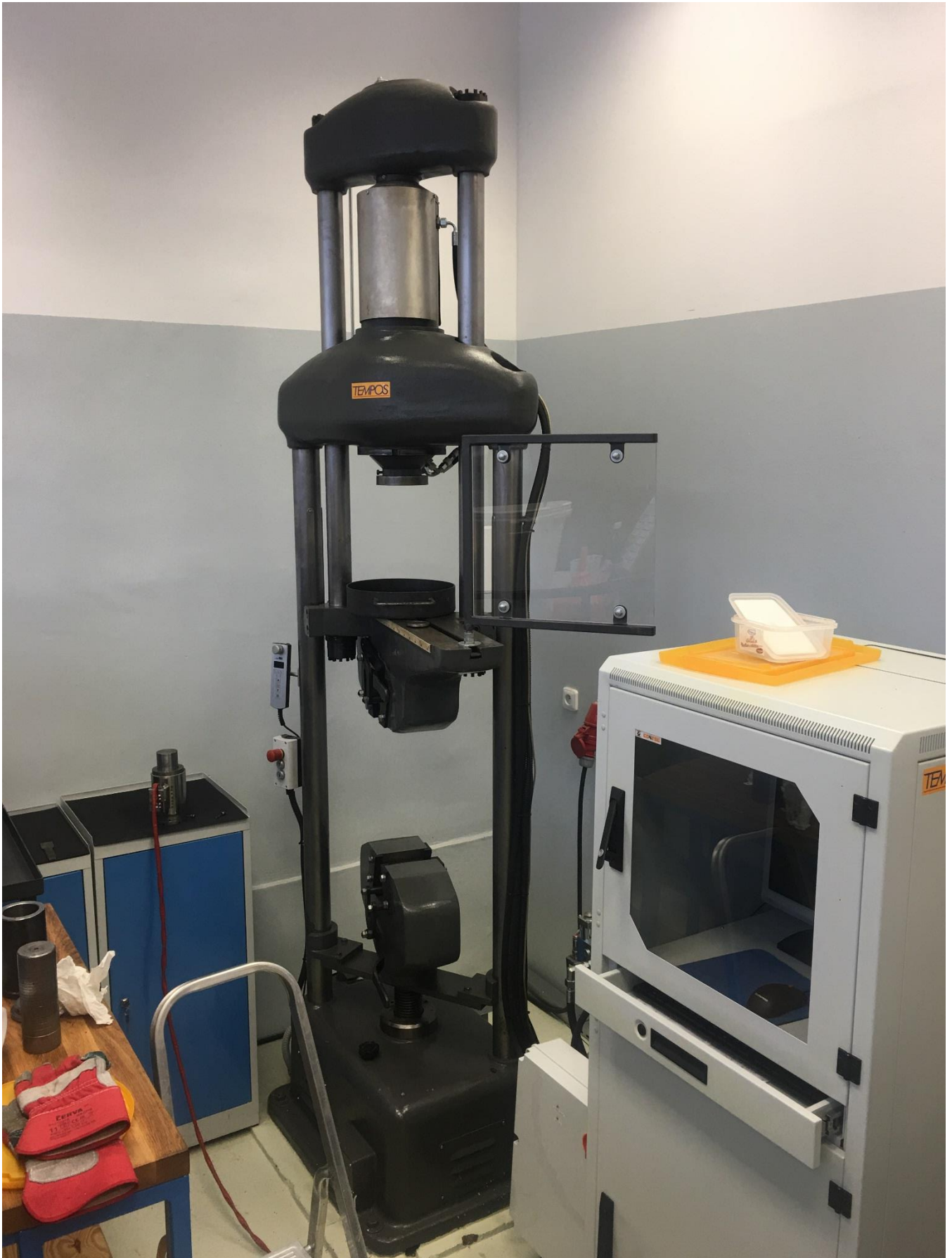
Figure 14. TEMPOS® ZDM 50 hydraulic press capable of creating a force of 500 kN
