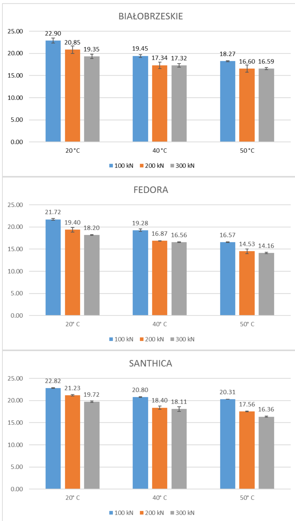
Figure 9. Residual oil (%) in hemp cakes of variety a) Białobrzeskie b) Fedora c) Santhica
