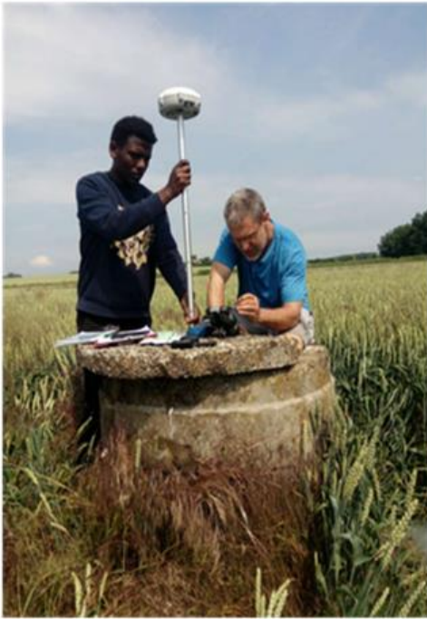
Figure 12: Reading the Exact localization of the control shaft by geodetical GPS. Source: Photo: K. Bářková; Scheme: V. David
