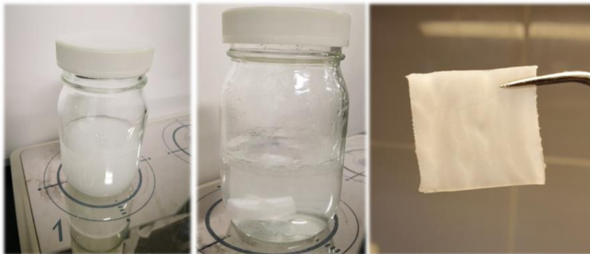
Figure 5-5 Preparation of PVA hydrogel samples
