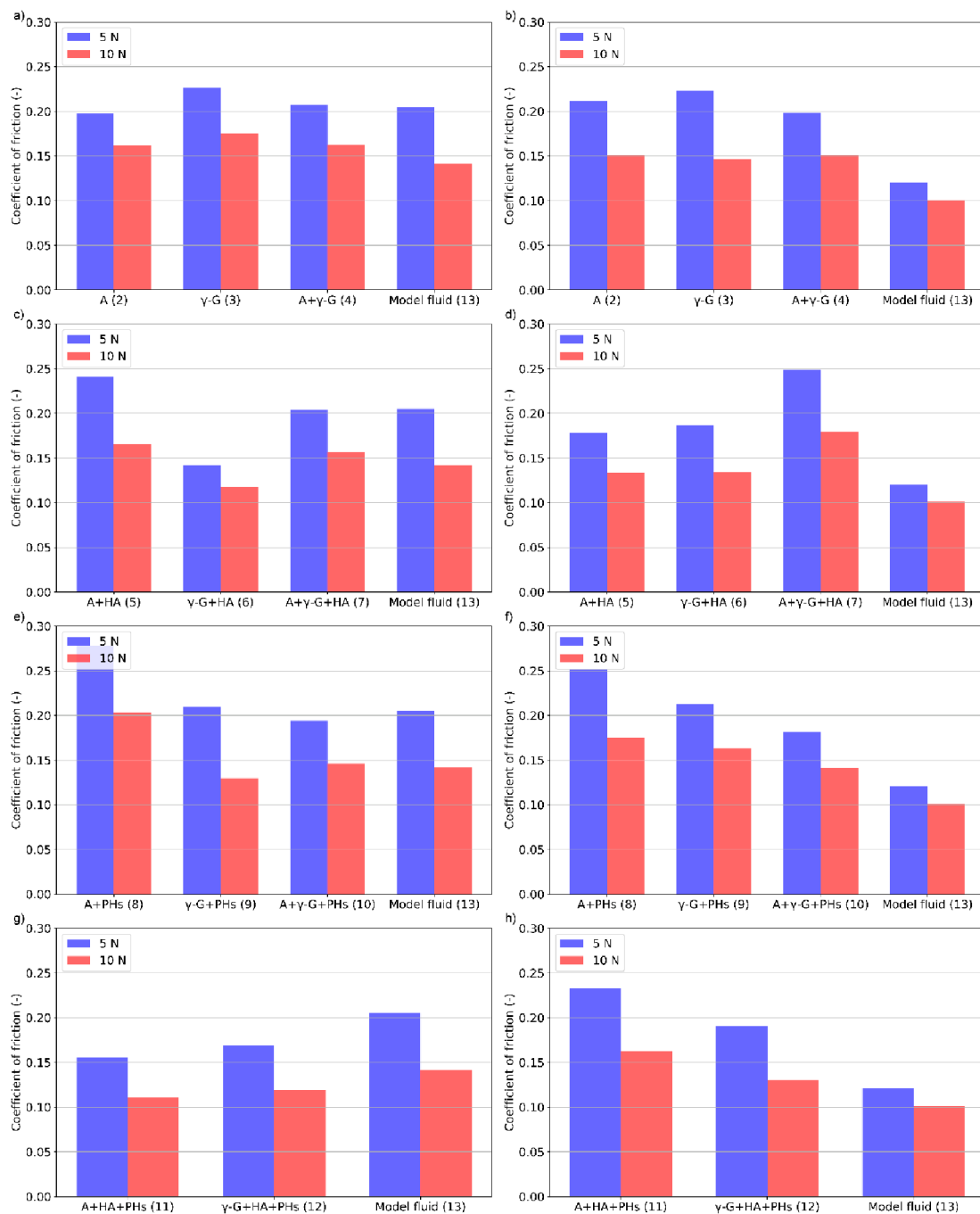
Figure 6. The effect of load on the friction coefficient for various protein- (a,b), HA- (c,d), PHs- (e,f), and HA + PHs- (g,h) based lubricants; PC (left) and OC (right).
