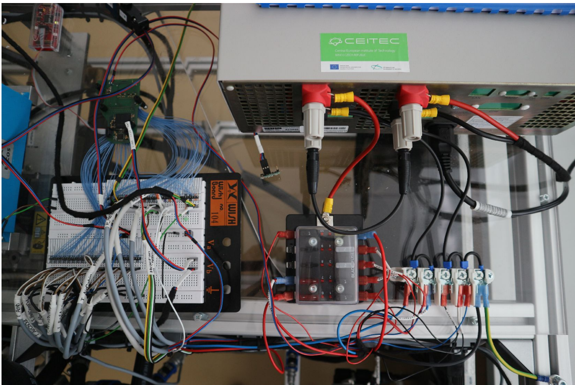
Fig. B.6: TEMCU, debug breadboard and 12 V power supply and fuse box
