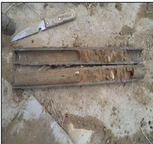
Figure 2.3 Field test (SPT)
