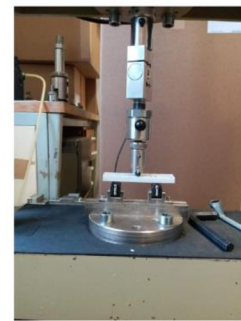
3-point bending test
