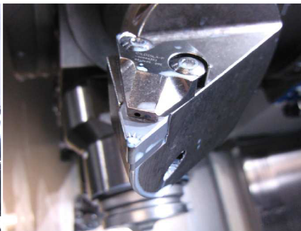
Obr. 35 držák JetstreamTooling (Seco-Capto C6-PDJNR-45065-15JETL)
