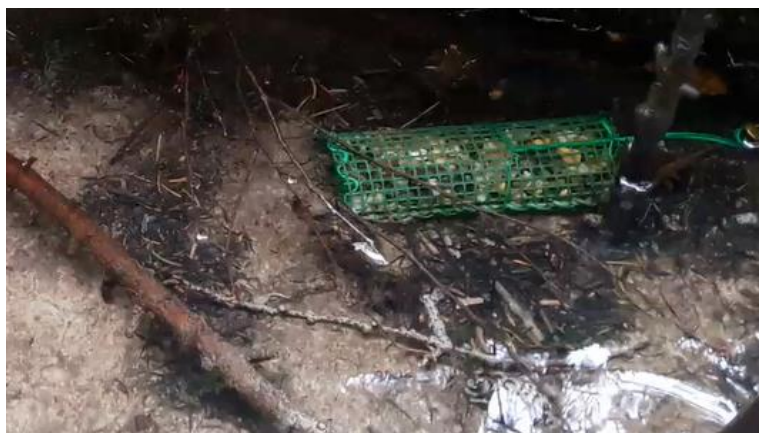
Figure 6: Artificial substrate cylinder installed for sampling biota as alternative method.
