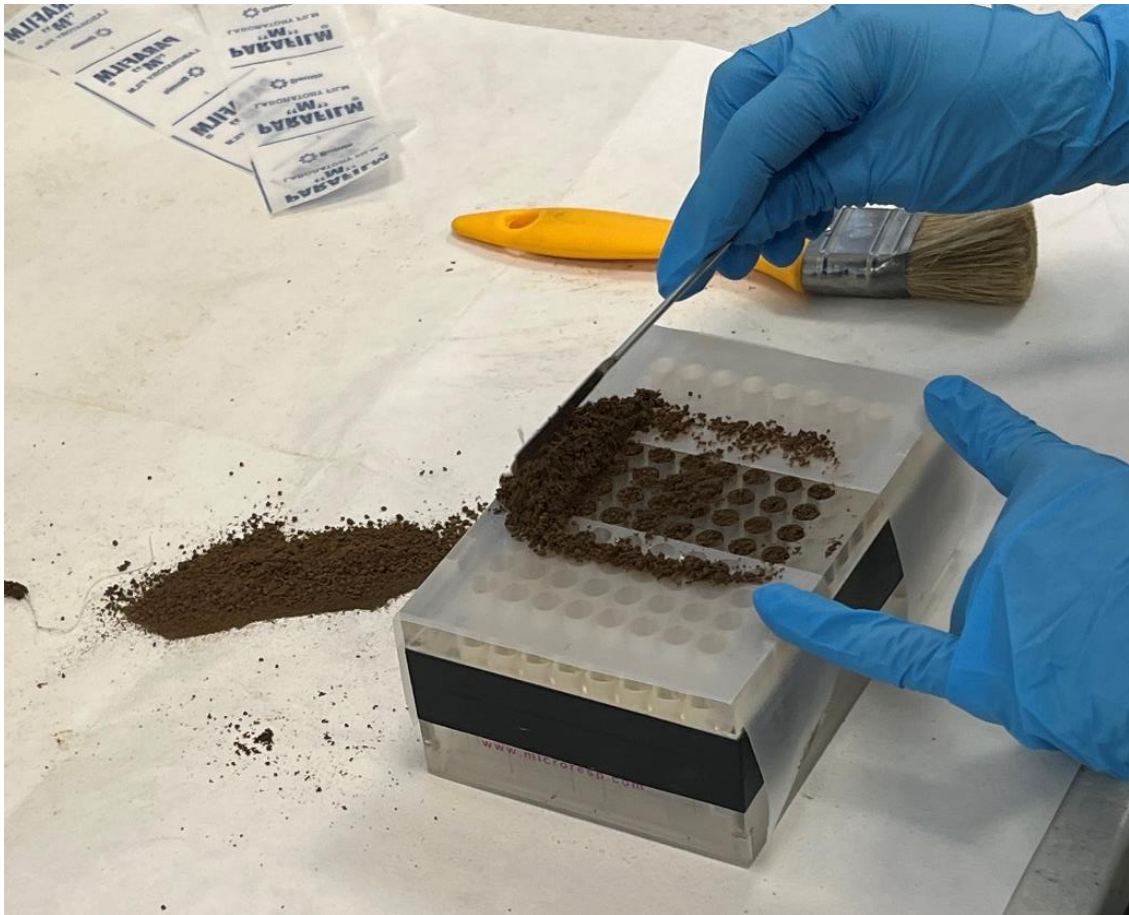
Fig. 7: Preparation of detection microplates.
