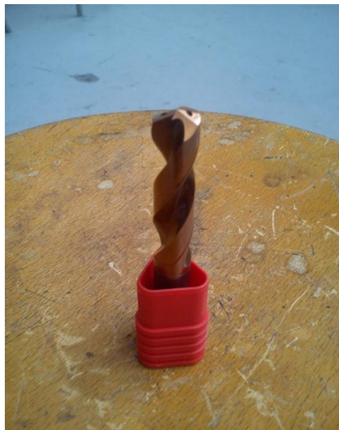
Fig. 4.20 – Twist drill R846-1200-30-A1A
