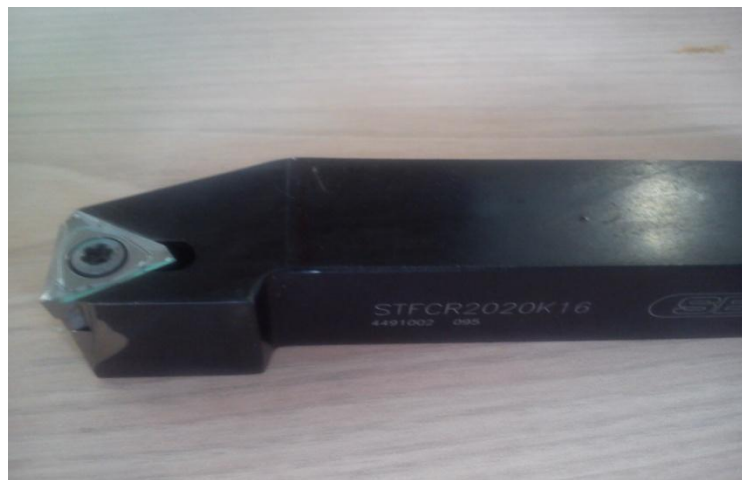
Fig. 4.10 – Cutting tool for EN-AW 7020
