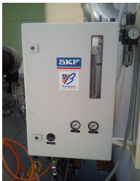
Fig. 4.16 - Numerically controlled MQL generator by SKF
