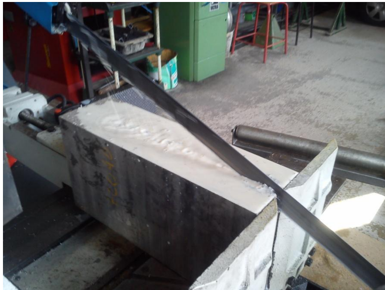
Fig. 4.11 – Band sawing of an aluminum alloy blank
