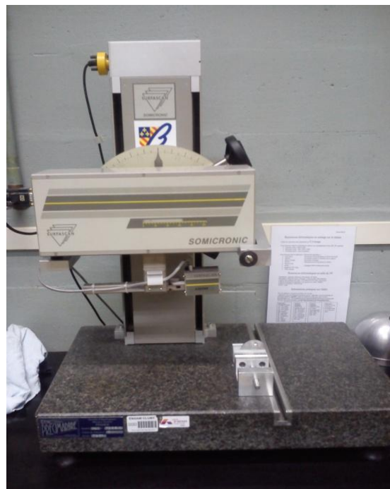
Fig. 5.3 Machine Surfascan for measuring of the surface roughness
