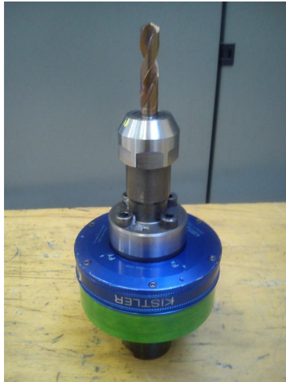
Fig. 4.17 - Rotary piezoelectric dynamometer KISTLER 9123C
