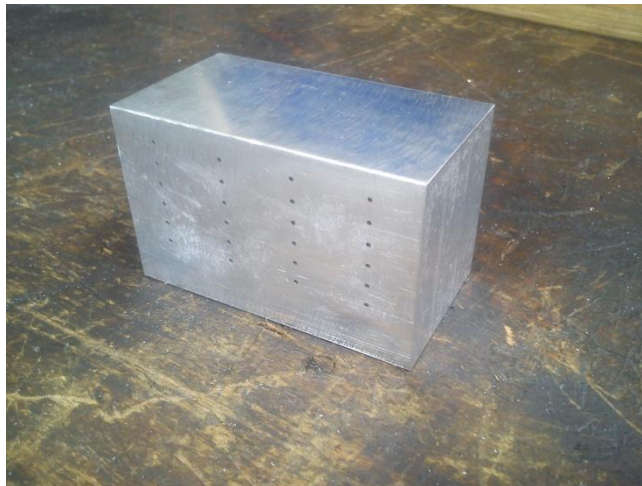
Fig. 4.12 – Workpiece for the drilling test
