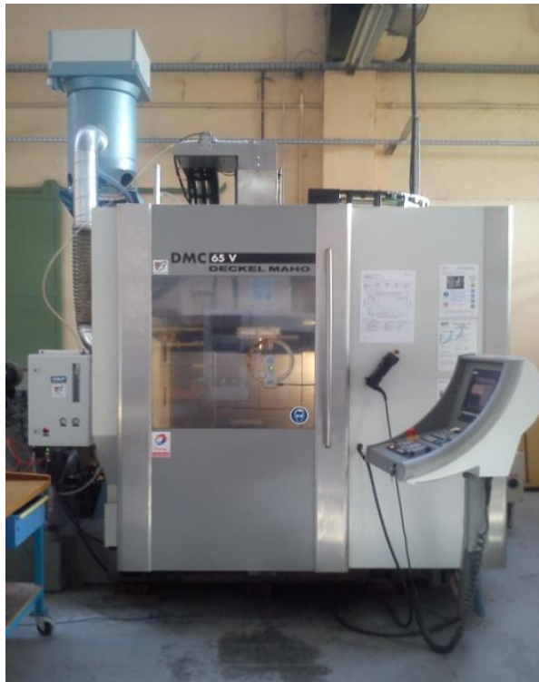
Fig. 4.15 - CNC 3-axis milling machine DMG DMC 65V.
