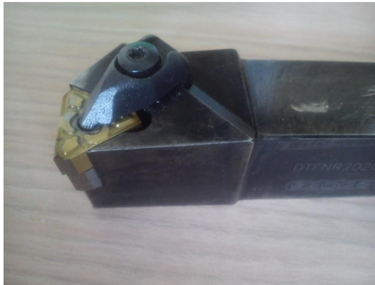
Fig. 4.9 – Cutting tool for AISI 316L
