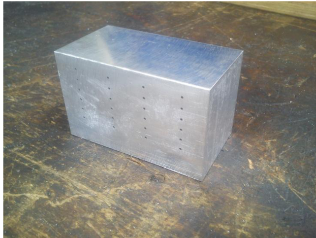
Fig. 4.12 – Workpiece for the drilling test
