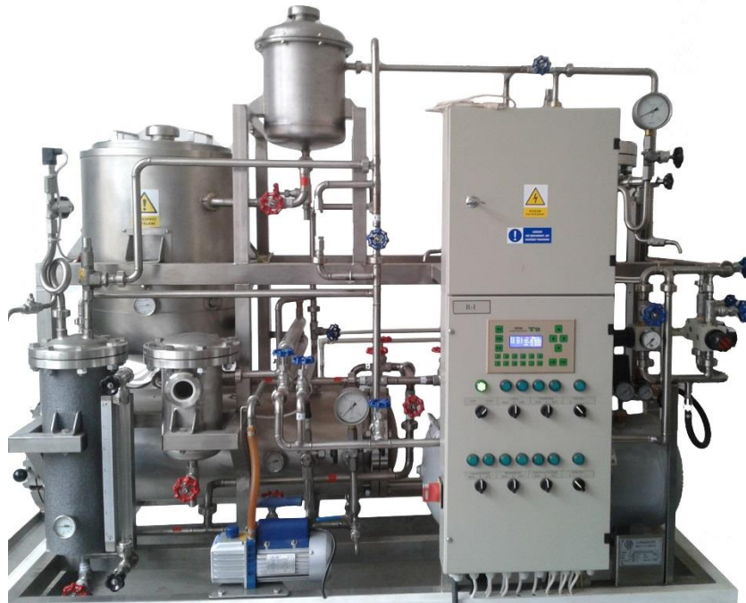
Figure II. 1 Vacuum-pressure impregnation equipment: JHP 1-0072
