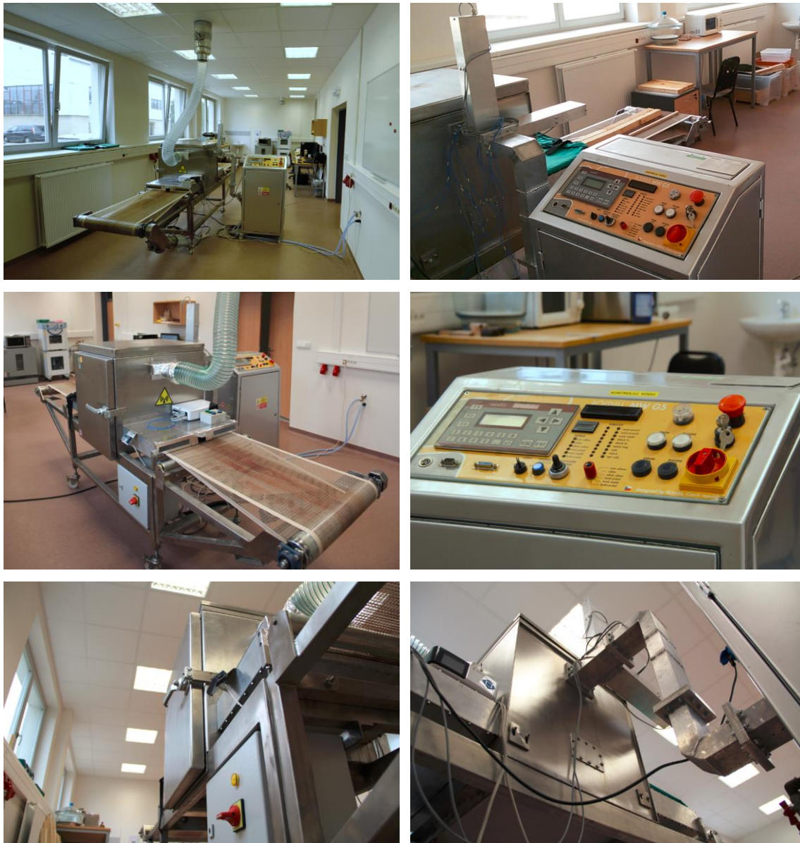
Figure 4 Continues MW device – basic view of conveyor, generator, modification chamber and waveguide
